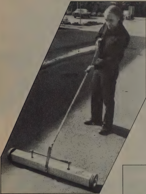
↑ Magnetic sweeper grabs ferrous tire-nabbers outta the driveway or even your lawn. A pull on the handle releases the gathered material, in this case a nail, a paperclip, and a rusty razor blade ($6/day).
